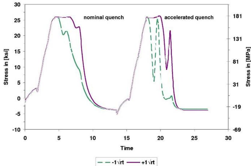
Figure 1 Axial Stresses at Shell ID due to Axial Temperature Gradients
